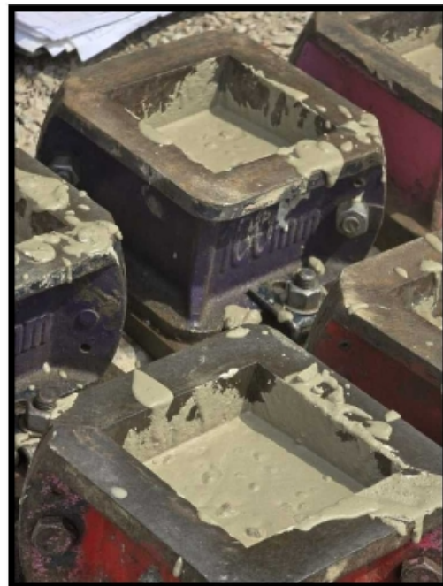
Concrete cubes which will be tested in a range of conditions.
