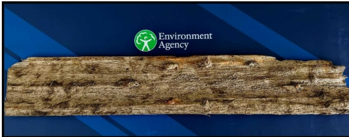
Timber plank from the upstream apron of Grand Sluice.
